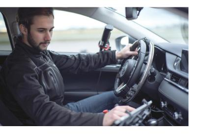
The **DRc** is also characterized by its compact design that frees up space and enables quick and hassle-free installation. The steering and throttle/brake robots are interconnected to provide ample room for electronics and data acquisition systems as well as easy access for test engineers. In addition, the **DRc** Box, contains all electronic components, which can be easily installed with ISOFIX in the rear seats.
